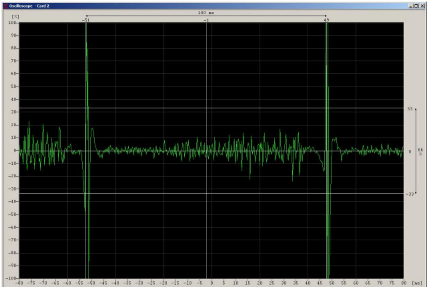
Chinese broadband OTH radar – The radar sound was similar to a woodpecker caused by the narrow filters in amateur transceivers.
