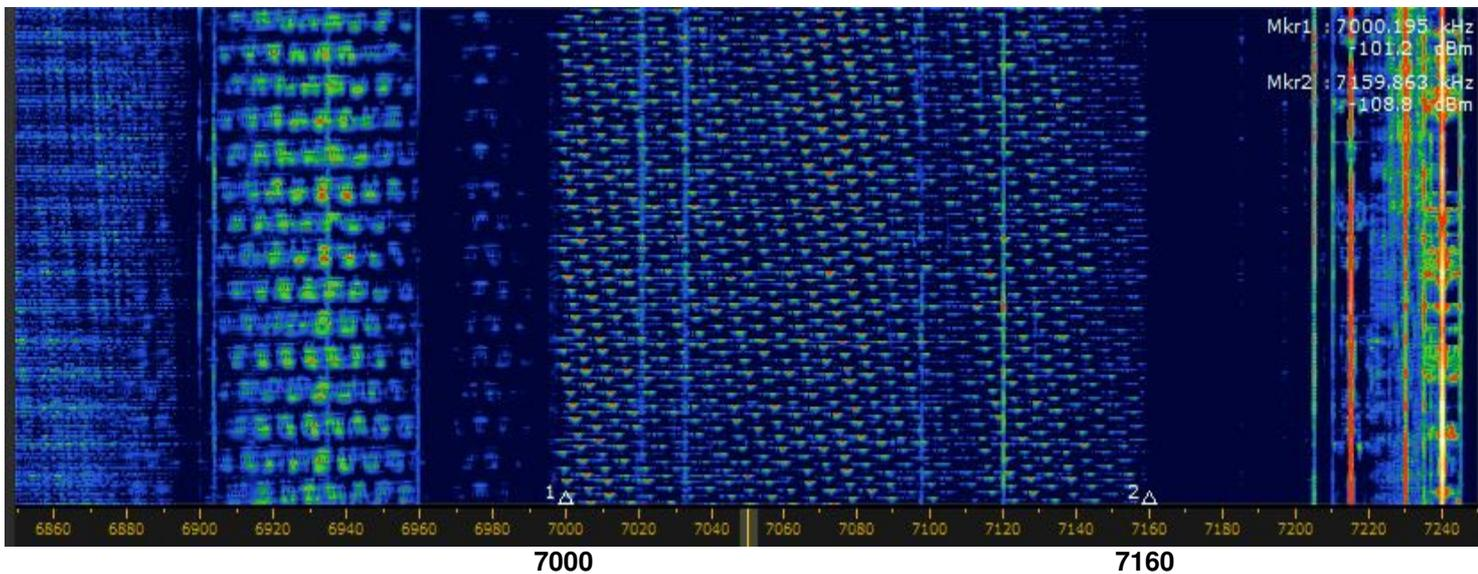
Measuring the sweeprate (PRF) with the W-Code oscilloscope function – 100 msec between the sweeps
